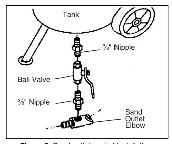
Figure 2. Sand outlet control installation.
